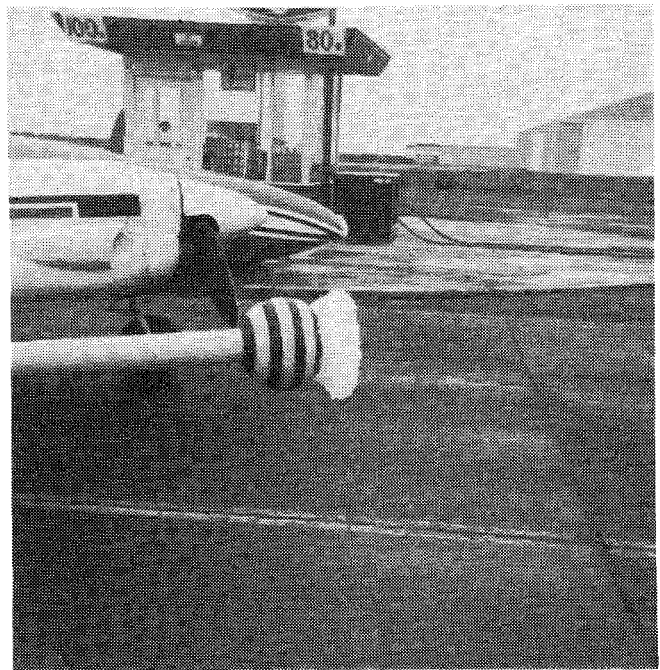
Fig. 7 Ice accretion on spherical probe.
